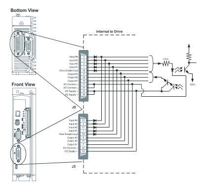
Figure 19: Epsilon I/O to Command Connector Internal Connections
